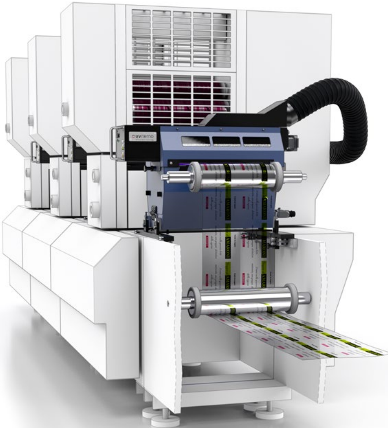
Fig. uviterno SRK units; temperature-sensitive application when printing on thin films.
